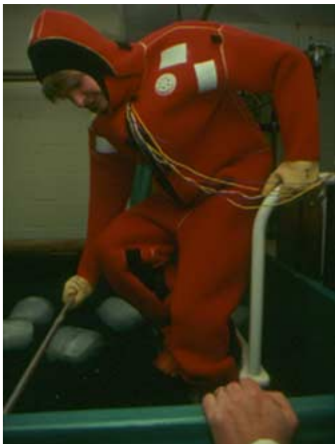
Fig. 17-7. This flotation survival suit has hypothermia protection capabilities. Note that the gloves, feet (not shown), and hood are part of the suit, and are intended to keep water entry down to a few cubic centimeters. The subject is entering a tank with the water temperature set at 0°C, in a 2-phase system. Core temperature data from this garment are presented in Figure 17-8.
